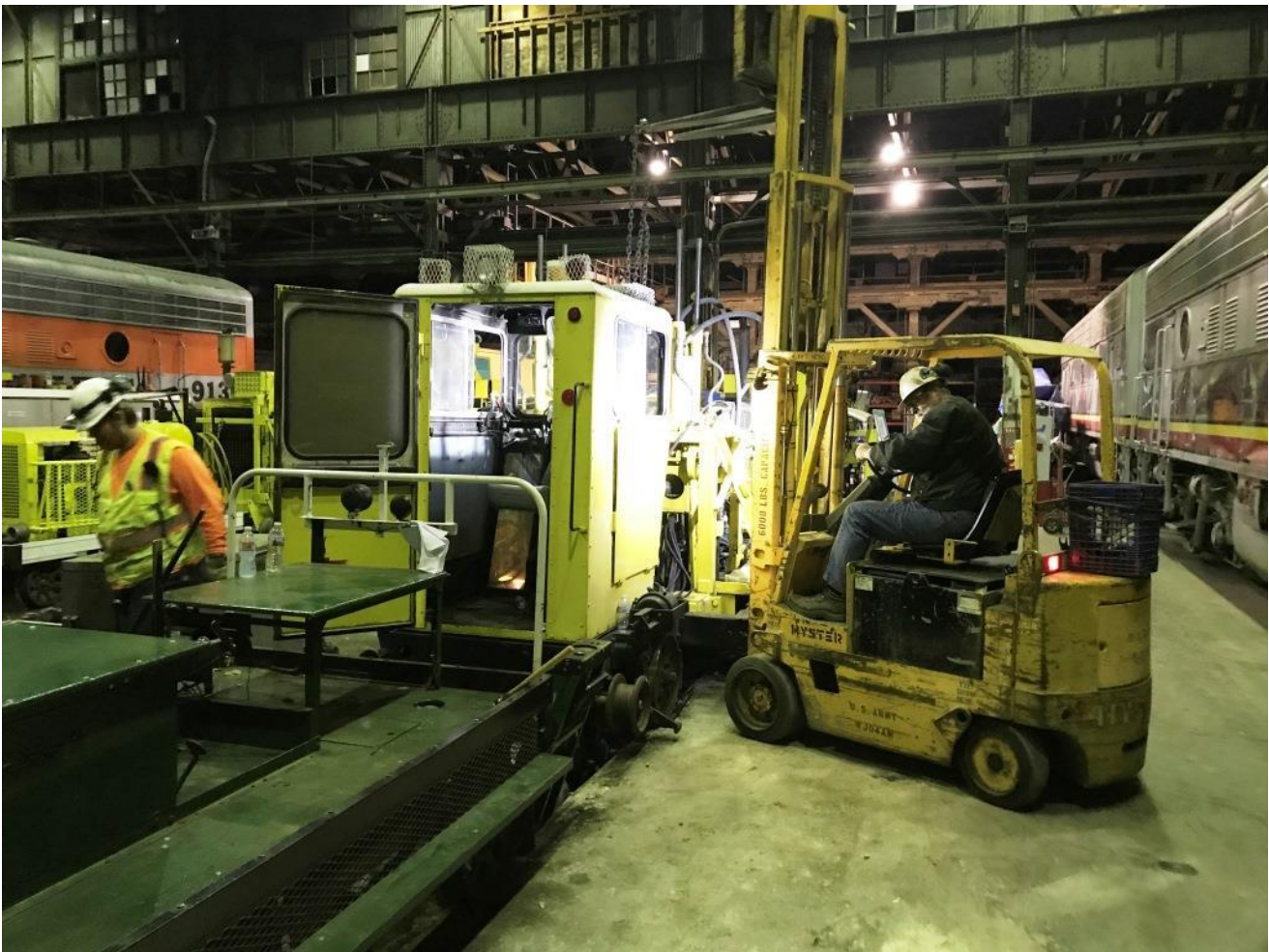
Alan on the forklift suspends the weighty hydraulic cylinder so that it can be connected from beneath
