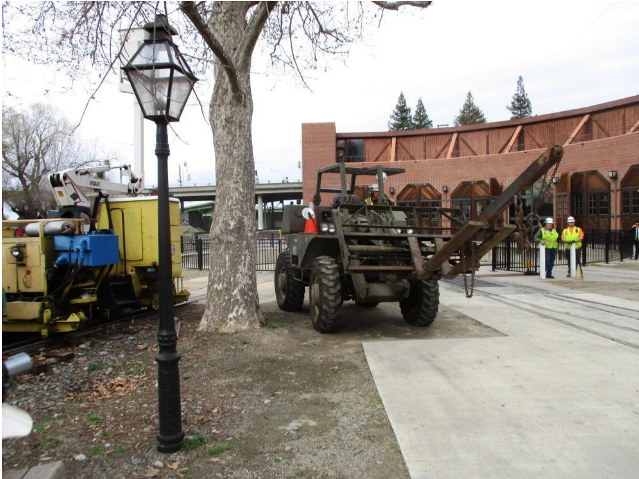
One last task for GM2: take the "stinger," which we use to lift sticks of rail, back to the Shops
